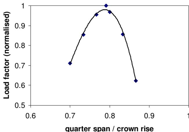
**Figure 8 Influence of varying  $\frac{1}{4}$  and  $\frac{3}{4}$  point rises (as ratio of midspan rise)**
