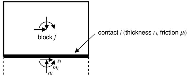
**Figure A1-1 Block and contact forces**
