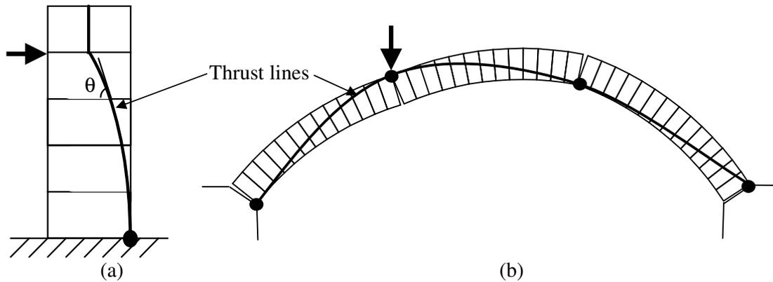
**Figure 2 Thrust line at collapse in (a) masonry pier, and (b) masonry arch**
