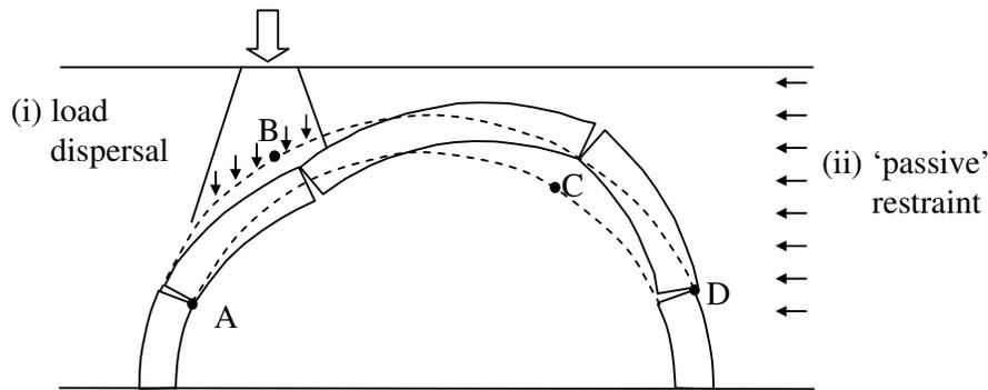
**Figure 5 Masonry bridge soil-structure interaction**
