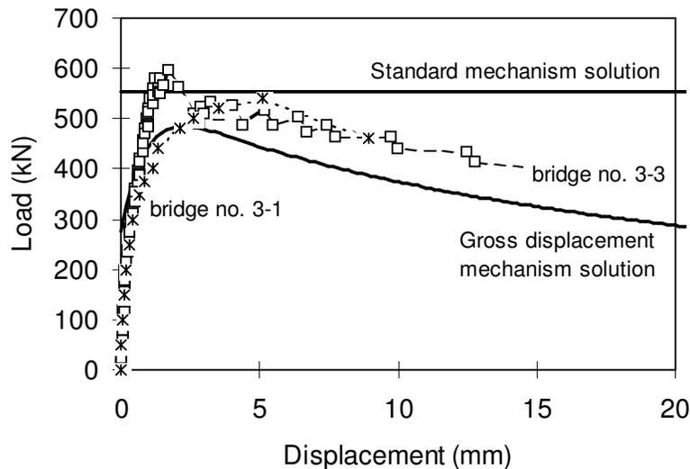
**Figure B-2** Experimental and predicted load vs. displacement response of single-span bridges
