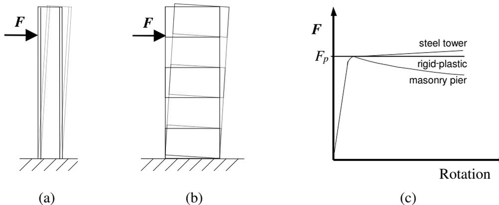
**Figure 1** Laterally loaded (a) steel column, (b) masonry pier, and (c) idealised response curves
