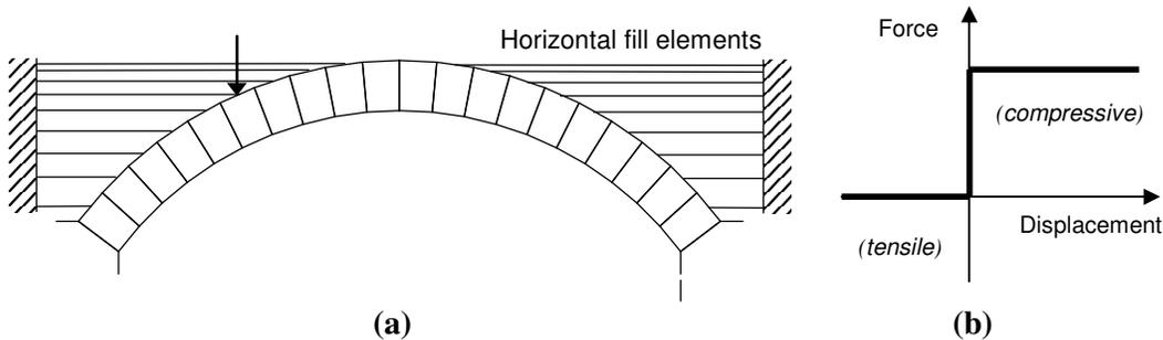
**Figure 7 Arch restrained with uniaxial fill elements (a), and (b) fill element response**
