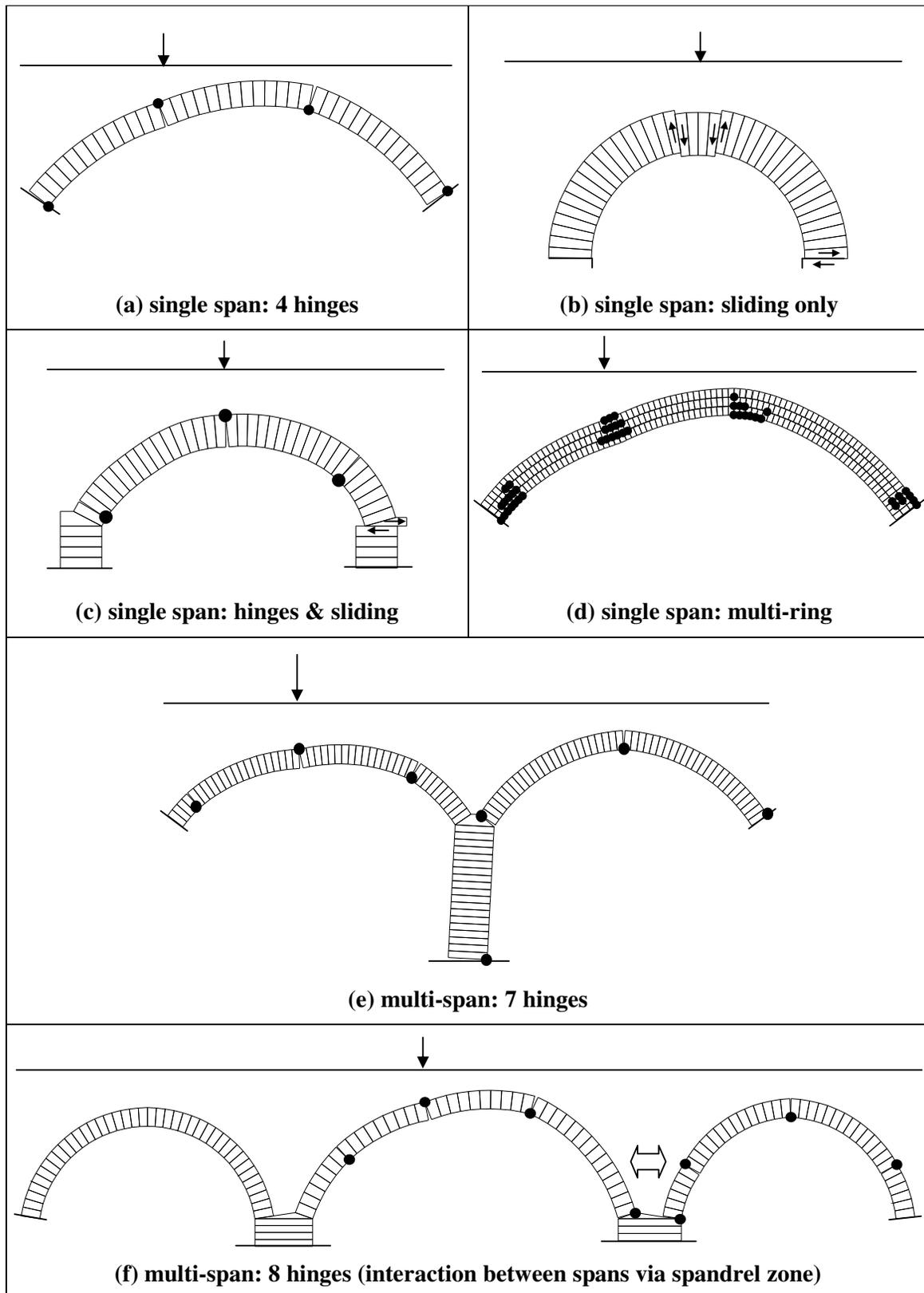
Figure 3 Selection of potential failure modes identified by RING
