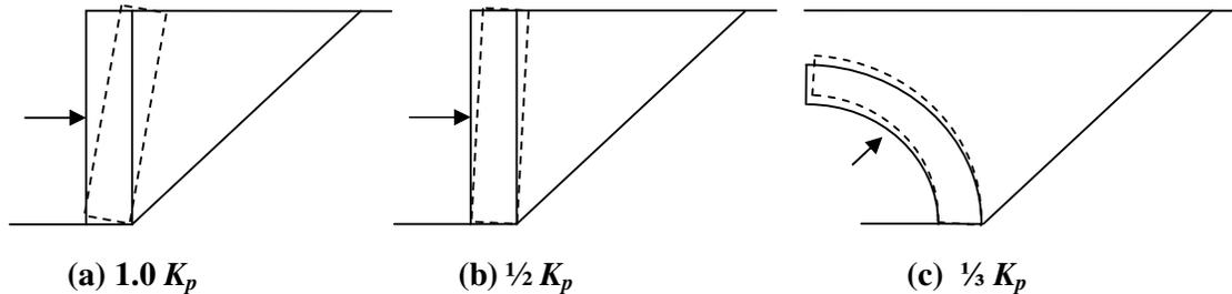
**Figure 6 Commonly used horizontal earth pressure coefficients: (a) large wall rotation, (b) small wall rotation ( $\approx 0.5\%$ ), (c) arch segment rotation into surrounding fill**
