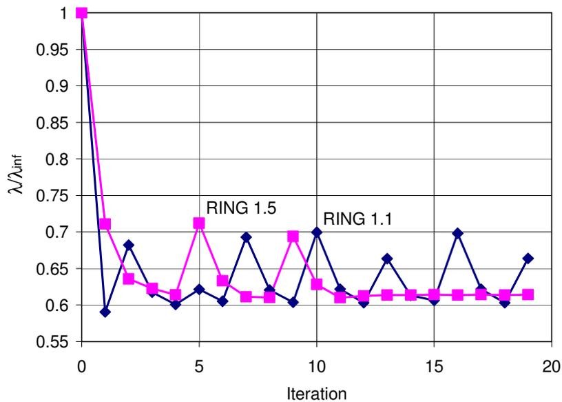
**Figure A2-1 Sample convergence characteristics for a multi-ring arch problem**
