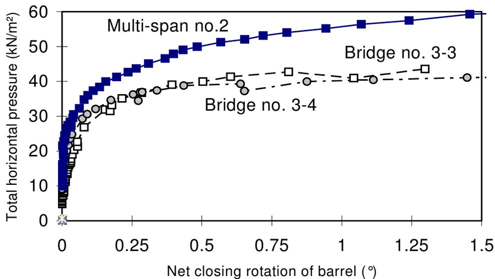
**Figure B-1 Mean horizontal backfill pressure vs. net closing barrel rotation of arch barrels**
